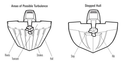
• As a general rule, the faster the boat can travel, the further aft and closer to the centerline of the hull the transducer has to be located in order to remain in contact with the water at high speeds.
